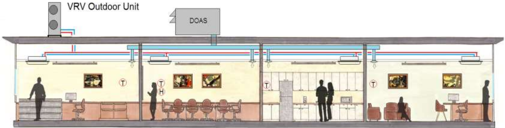
Typical Dedicated Outside Air System Installation
