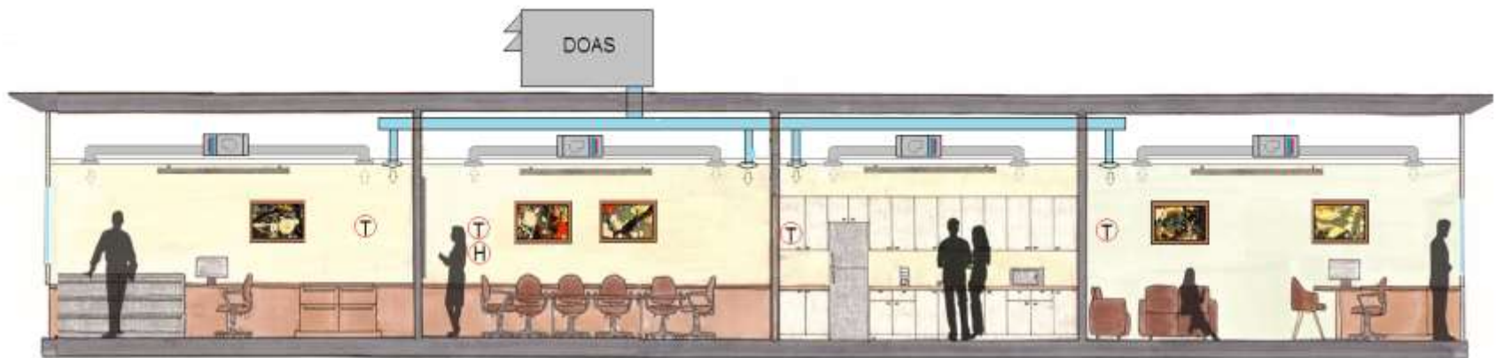
Typical Dedicated Outside Air System Installation
